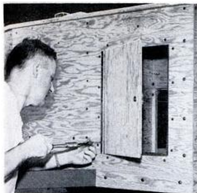
Lock-fitted, rubber-sealed doors to storage compartments in nose of trailer are hinged with piano hinges
